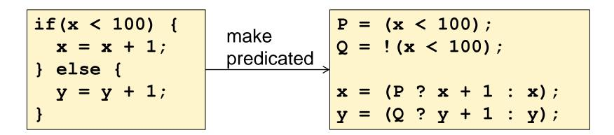
Apply **predication** to kernel so that at every execution point there is a predicate determining whether each of the threads are enabled
