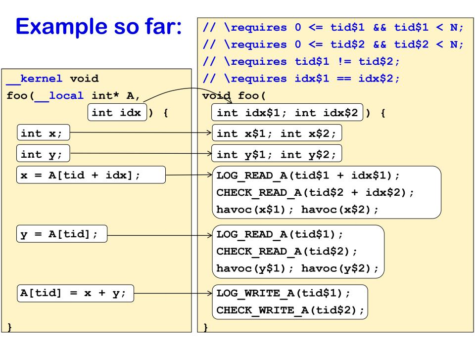
Global variables **READ\_HAS\_OCCURED\_A** and **READ\_OFFSET\_A** collectively log either **nothing**, or the offset of a **single** read from A by the first thread
